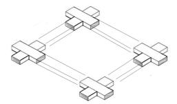
If the joints are marked and cut accurately, with a snug fit, there should be no movement once the pieces are engaged, thus holding everything in place without clamps.
