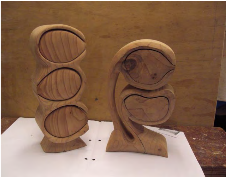
Two boxes almost finished with drawer pulls yet to be attached. It is interesting to see Sam's use of the grain in the draw fronts.
