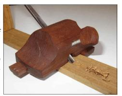
There is a slide on the base that can take a guide for edge use or a blank for wider use.
