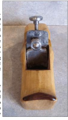
The adjuster was made from a metric bolt, turned down on my wood lathe. The tread on the adjuster has to fit smoothly into the threaded rod. Easier said than done. A digression was the need to research, manufacture and learn to use hand held metal cutting tools. A big solid lathe and a three jaw metal turning chick are essential. I turned a knob for the adjuster and silver soldered it on.
