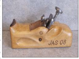
My solution was to convert a plane, made several years ago, by adding a blade up and down adjuster and a new lever cap to lock the blade in place. I probably should have started with a completely new plane as it would have been much easier. The job was complicated because I didn't know how to go about it and my metal working skills are limited. I had to invent processes as I went along. As a result practically every part was made twice.
