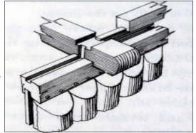
tongued into a grooved wall plate, and housings to the roof collar ties. Remains of small narrow adzes were found, tat were likely used to form the grooves..
