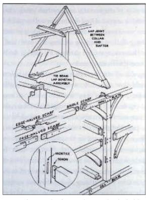
works 'structurally'. Basically it is set of triangular forms, that work a little like an angled truss.
