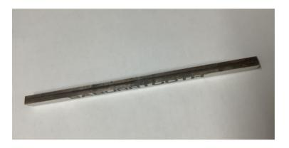
Above is a carpenter's pencil that I have sanded down to expose the lead, making sure that it is straight. I then use this when I am turning to expose high spots on the outside of cylinders or the base of a bowl. Simple but effective.
