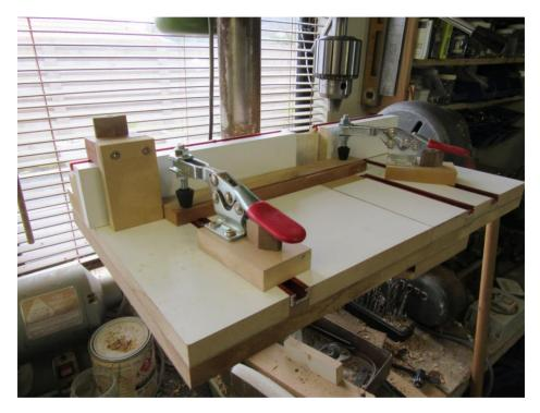
nuts embedded. The table is mounted on the round drill press base with 3 toggles allowing it to be aligned in many ways by rotating or offsetting the cast drill table
