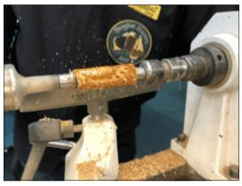
have using thin CA glue to ensure it soaks into the fibres. I probably overuse the accelerant to Pastensure the gaps are filled by the glue. Take care, and remember you need to <u>put the blank down</u>.
